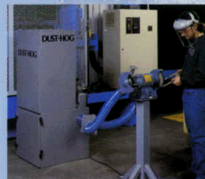
Airborne grit, fibers and rouge powders are eliminated when a buffing station is ducted to a Supra-Conic SC600.
