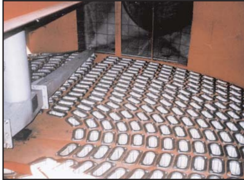
Filter tubes in the RF filter are arranged in non-aligned concentric rings, providing more filter cloth in less area since the nozzles on the traveling air plenum do not touch the filter tubes, the need for tight alignment tolerances and the possibility of tube damage are eliminated.
